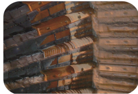
F.E. composite liners on \Phi 10.37 \times 5.19\text{m} SAG mill
