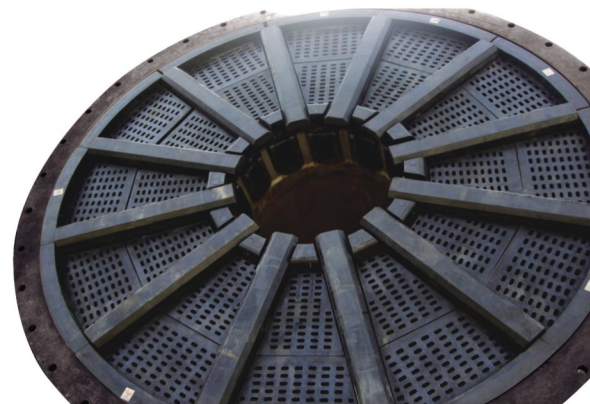
D.E. rubber grates on \Phi 3.2 \times 4.5\text{m} ball mill
